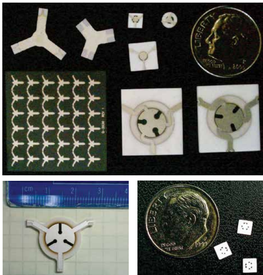
Figure 5. Photographs of integrated cofired mm-wave circulator devices.
